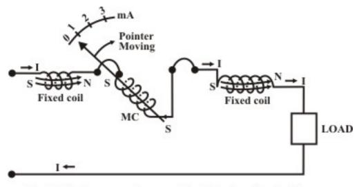
Fig. 43.2(a): Torque produces positive deflection (clockwise)
