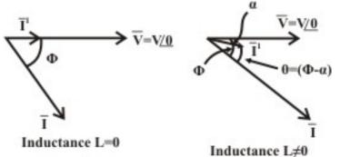
$I_1 I_2 \cos \theta$ , where  $I_1$  and  $I_2$  are r.m.s values and  $\theta$  the phase angle between the two currents (pressure coil current and current coil current). The current through moving coil  $I = \frac{V}{R}$ , is in the same phase as that of load voltage, where *R* is the resistance of a non-inductive voltage–coil circuit. Then  $\theta = \phi$ , load phase angle.
