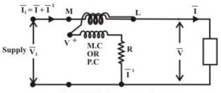
Fig. 43.8(a): Compensated wattmeter
