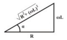
$$T_{\text{instantaneous}}(t) = I_{\text{m}} \sin(\omega t - \phi) \frac{V_{\text{m}} \sin(\omega t - \alpha)}{\sqrt{R^{2} + (\omega L)^{2}}} \frac{dM}{d\theta}$$
