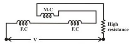
Fig. 43.5: Electro-dynamic voltmeter connection
