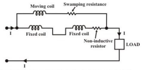
Fig. 43.4: Electro dynamic Ammeter (above 250mA) connection
