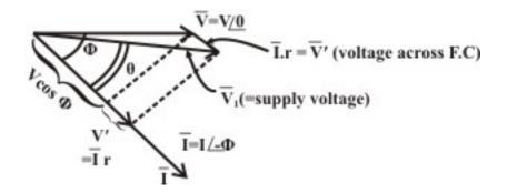
where V' is the magnitude voltage across the current coil or fixed coil.
