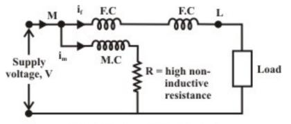
Fig. 43.6: Wattmeter Connection
