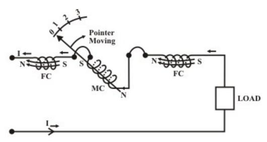
Fig. 43.2(b): Current flowing right to left produces positive deflection again.
