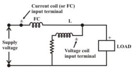
Fig. 43.8(b): Wattmeter terminal connection
